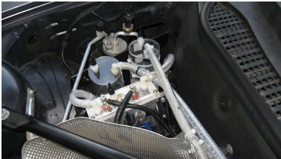
HH2 install To Bubblers shown
