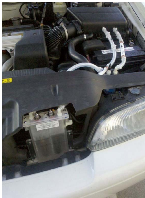
HH2 system fitted
