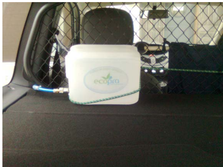
Ecopra Component – Water reservoir
