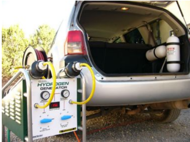
United Nuclear's Solar Hydrogen fuelling station - Source
